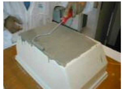
Dé-bullage du gel coat. Out gazing of the gel coat.
