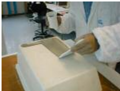
Application et dosage du gel coat. Application of the gel coat.
