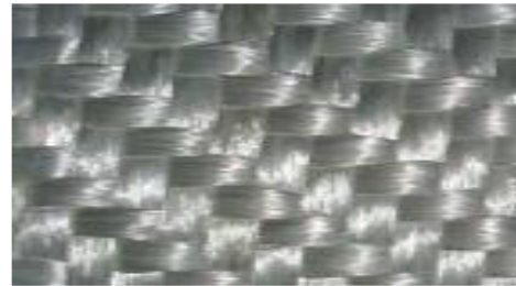
Fig. 12 : Twill weave (Twintex® 1-1, 745 g/m 2 or 1485 g/m 2 , 60%).
