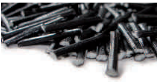
The front end of the Audi Q7 is made using OCV Reinforcements TWINTEX® long fiber pellets (Plastic Omnium Auto Exterior, France)
