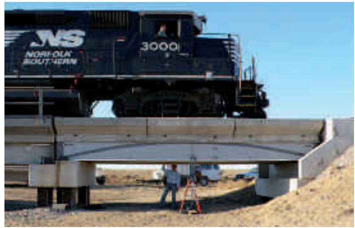
A full-size locomotive pulls 26 heavy axle-loaded coal cars 30 feet without incident
