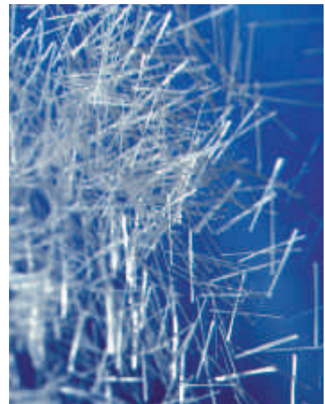
OCV Reinforcements specialty AR glass is used in glass-fiber reinforced concrete
